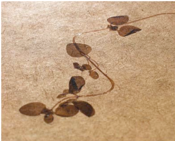
Figure 5: Real flowers were pressed into the material and became embedded into the hardboard
