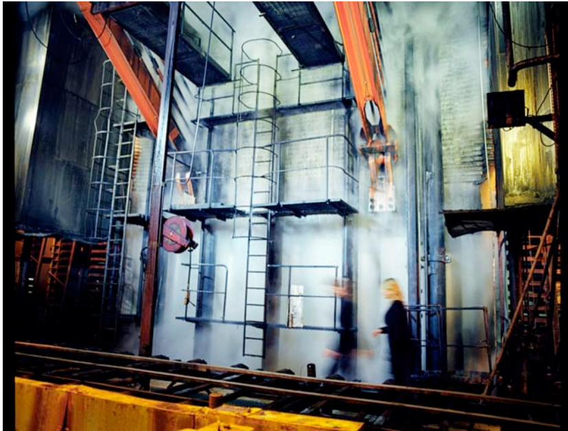
Figure 4: The huge Masonite press were the chips exploded under a steam pressure of 1000 pounds per square inch.
