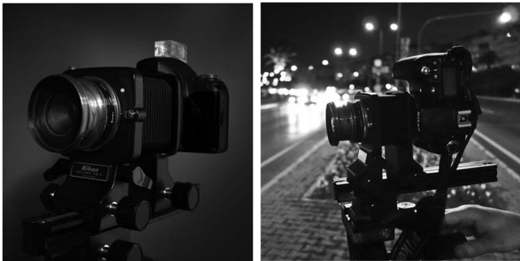
Figure 4 shows the hybrid camera consisting of a 19 th century British lens and contemporary prosumer Digital SLR body.
