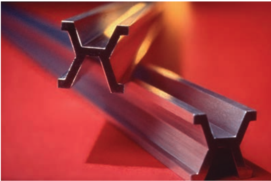
Figure 1 shows two international prototypes of the meter. Notice the “Tresca sections”. Source: Wikipedia.
