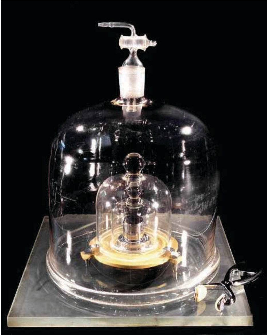
Figure 3 shows the IPK, the international prototype of the kilogram as it's kept at BIPM. Source: BIPM.
